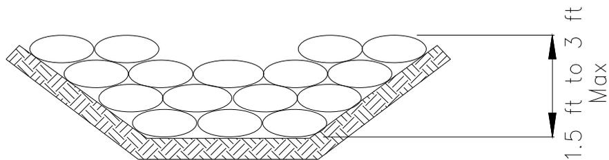
GRAVEL BAG CHECK DAM ELEVATION
